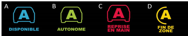
Figure 2. Pictograms displayed on the HMI: A: autonomous driving available; B: autonomous driving activated; C: take-over request (8s); D: take-over request (45s)
