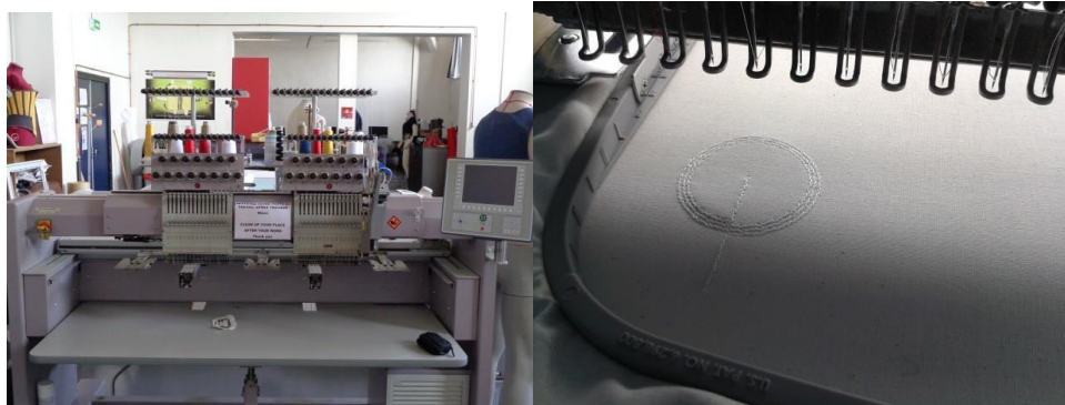
Figure 1. Photography of the ZSK embroidery machine (a) and a zoom on needles during an embroidery process (b).
