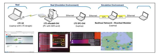
Fig. 2 OAI platform and screen shots showing UE and eNodeB interaction
