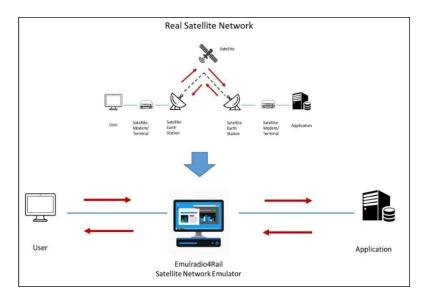
Fig. 6 Solution for the Satellite Network Emulation
