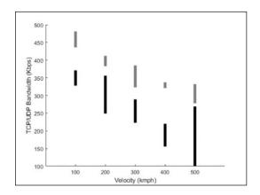
Fig. 5 TCP (black bars) and UDP (gray bars) bandwidths variation in terms of the vehicular speed
