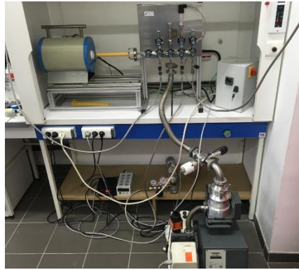
Fig.1 – Overview of the original isotopic exchange device for operating up to P = 50 bar and T=1100^\circ\text{C}
