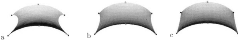
Fig. 6. Combination of SSDM and FDM for different values of coefficients a) q_{sj} = 1 and q_{lj} = 6 b) q_{sj} = 1 and q_{lj} = 25 c) q_{sj} = 1 and q_{lj} = 100
