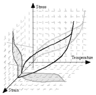
Fig. 3. Stress-strain-temperature evolution during a pseudoelasticity test
