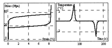
Fig. 5. Numerical stress-strain curve and temperature evolution in a pseudoelastic test
