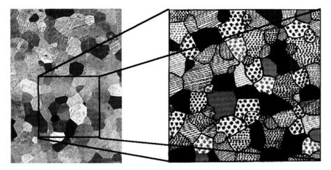
Fig. 6. RVE of a polycrystalline sample of CuZnAl SMA obtained by image analysis. Different patterns and colors stand for different crystallographic orientations
