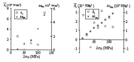
Figure 11: Average dissipation and thermoelastic sources amplitude for aluminium alloy
