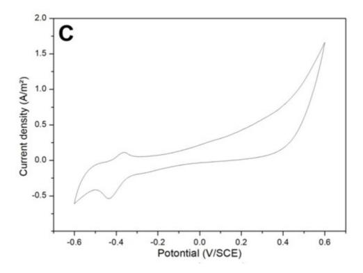
**Figure 4.** Cyclic voltammetries recorded using carbon felt in YPG liquid medium. A/ without methylene blue, B/ with methylene blue and C/ supernatant.
