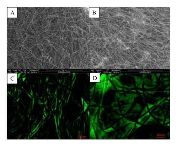
**Figure 5.** ESEM images of *Hansenula fabianii* bioanodes formed on carbon felt (A/ absence of methylene blue and B/ presence of methylene blue) and epifluorescence microscopy (C/ absence of methylene blue and D/ presence of methylene blue).
