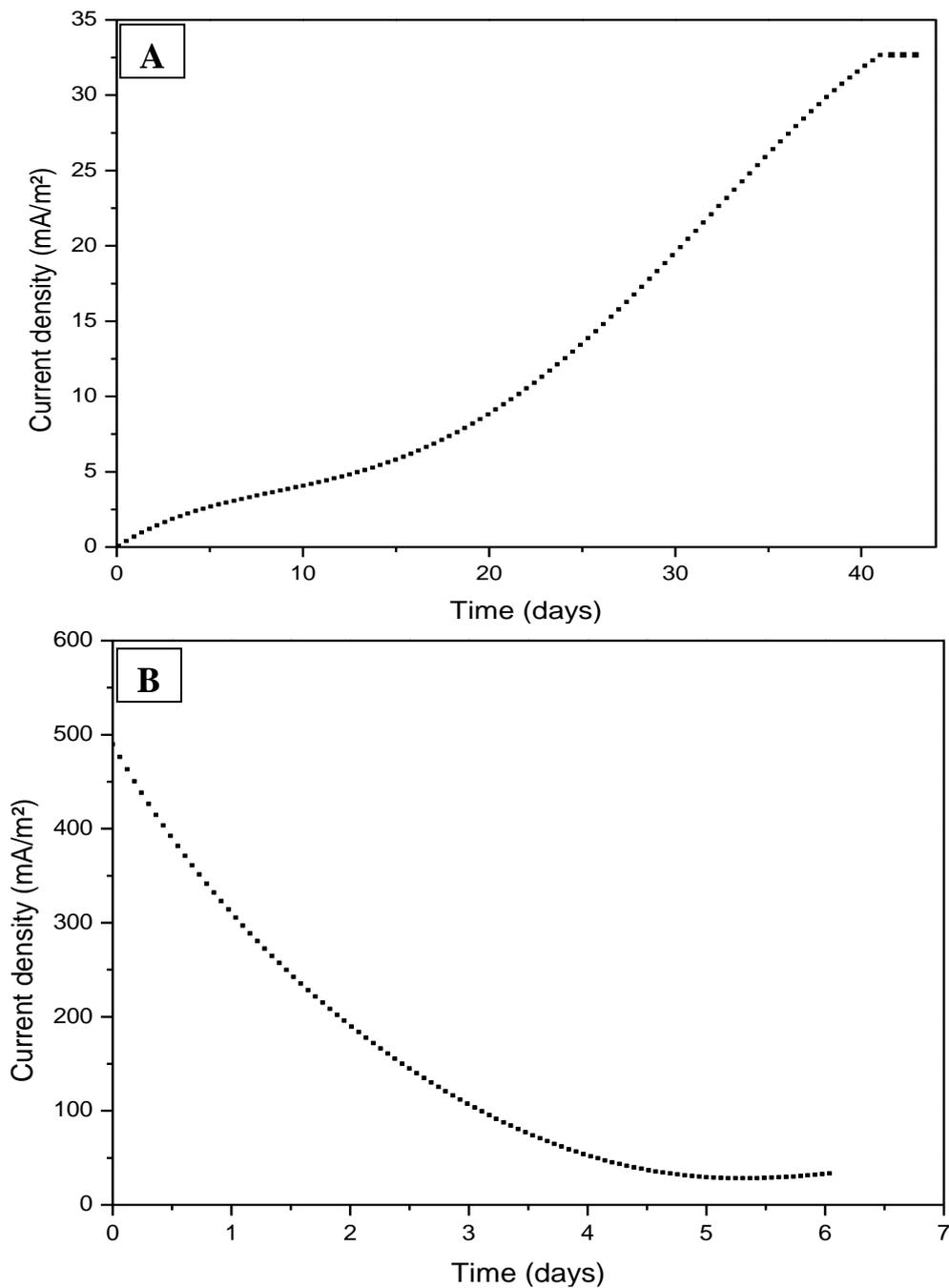
**Figure 3.** Evolution of the current density on carbon felt electrode polarized at -0.1 V vs. SCE in YPG liquid medium inoculated with *Hansenula fabianii* A/ without methylene blue and B/ with 300 mM of methylene blue.
