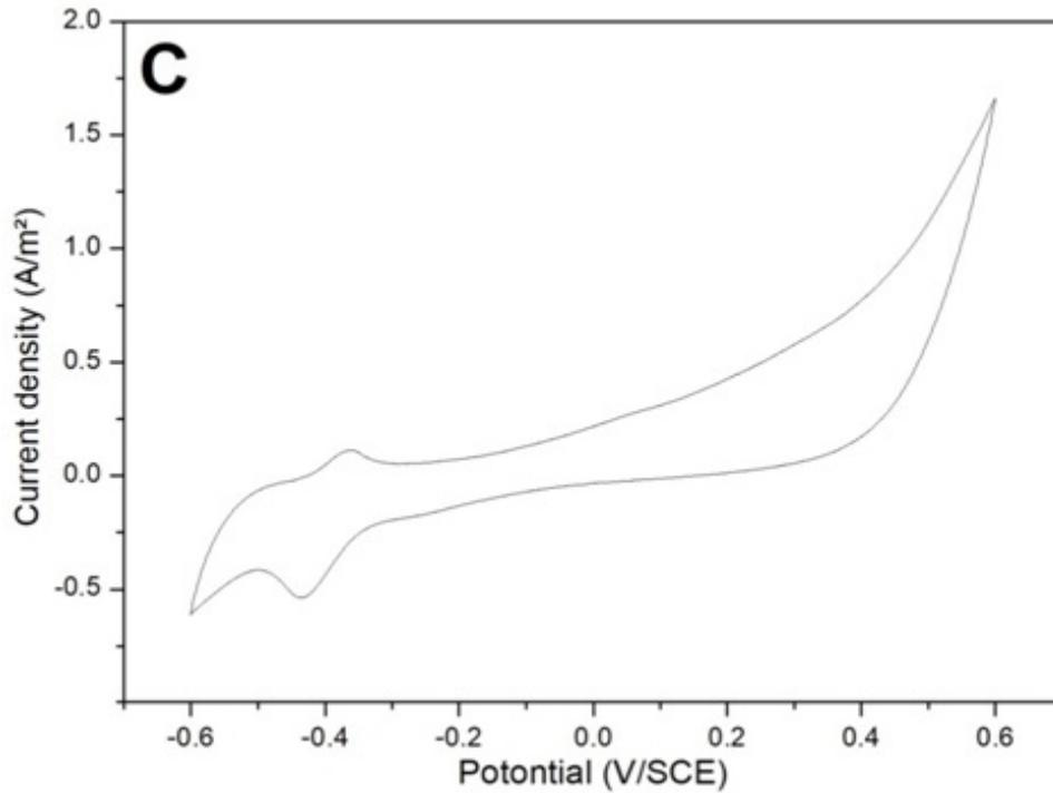
**Figure 4.** Cyclic voltammeteries recorded using carbon felt in YPG liquid medium. A/ without methylene blue, B/ with methylene blue and C/ supernatant.
