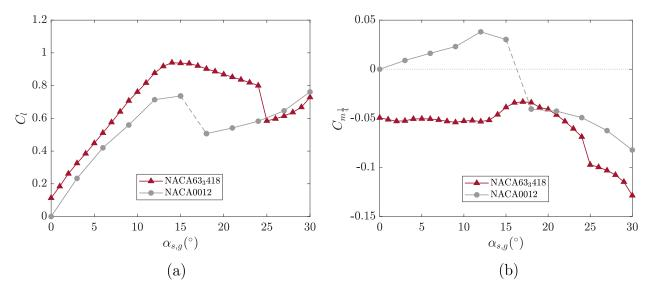
Fig. 2 Comparison of the (a) lift coefficients and (b) pitching moment coefficients at the quarter chord between the two NACA airfoils. The angle resolution being too poor to measure precisely the static stall angle for the NACA0012 airfoil, dashed lines where choosen around the stall angle in order not to mislead the reader.
