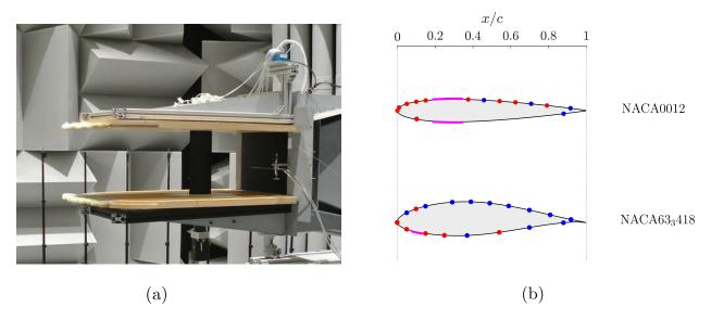
Fig. 1 (a) Picture of the nozzle exit (b) Schematic of the two airfoil shapes and positions of the surface pressure measuring points. Red dots and blue dots show the positions where only the steady-state surface pressure is measured and the positions where both the steady and fluctuating wall pressures are measured, respectively. Purple areas show the positions of the tripping tapes.
