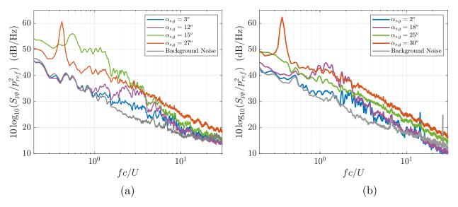
Fig. 5 PSD of far-field acoustic pressure for various static angles of attack and for (a) the NACA0012 and (b) the NACA63<sub>3</sub>418.
