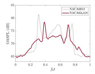
Fig. 11 Phase-averaged OASPL during the dynamic stall phenomenon for the two airfoils and k = 0.01.
