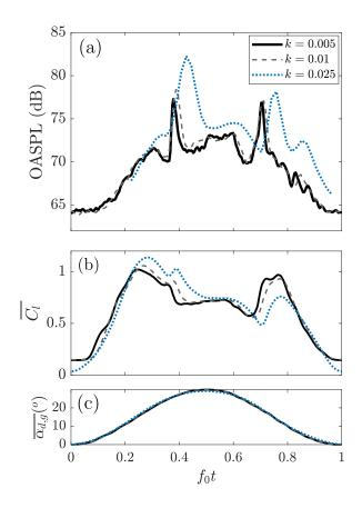
Fig. 10 Phase-averaged (a) OASPL, (b) lift coefficient and (c) angle of attack during the dynamic stall phenomenon for the NACA63<sub>3</sub>418 airfoil at various reduced frequencies. For the cambered airfoil and k = 0.025, the OASPL is cut for angles where the motor noise is dominating.
