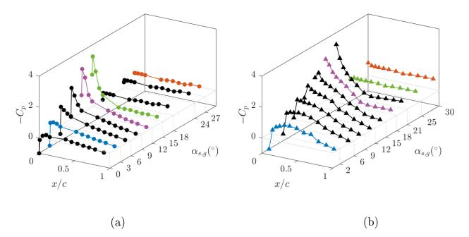
Fig. 3 Distribution of static pressure on the suction side of (a) the NACA0012 and (b) the NACA63<sub>3</sub>418 at various angles of attack. The colors correspond to the colors from Fig. 4 and 5.
