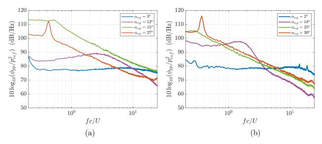
Fig. 4 Surface pressure PSD at x/c = 0.92 on the suction side for various static angles of attack and for (a) the NACA0012 and (b) the NACA63<sub>3</sub>418.
