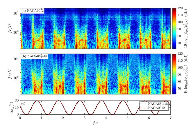
Fig. 6 Instantaneous spectrograms of surface pressure at x/c = 0.92 on the suction side for (a) the NACA0012 and (b) the NACA63<sub>3</sub>418, and (c) instantaneous angle of attack for  $\alpha_{d,g} = 15^{\circ} + 15^{\circ} \sin(2\pi ft)$  and k = 0.01.
