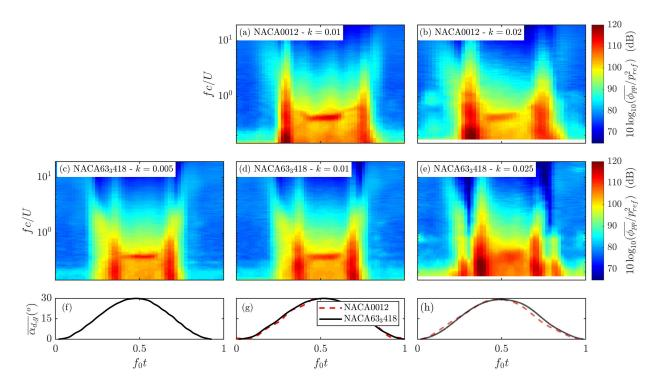
Fig. 8 Phase-averaged spectrograms of surface pressure at x/c = 0.92 on the suction side for  $\alpha_{d,g} = 15^{\circ} + 15^{\circ} \sin(2\pi f_0 t)$  for (a-b) the NACA0012 airfoil and (c-d-e) the NACA63<sub>3</sub>418 airfoil, and (f-g-h) phase-averaged angle of attack. The overbar denotes phase-averaging.
