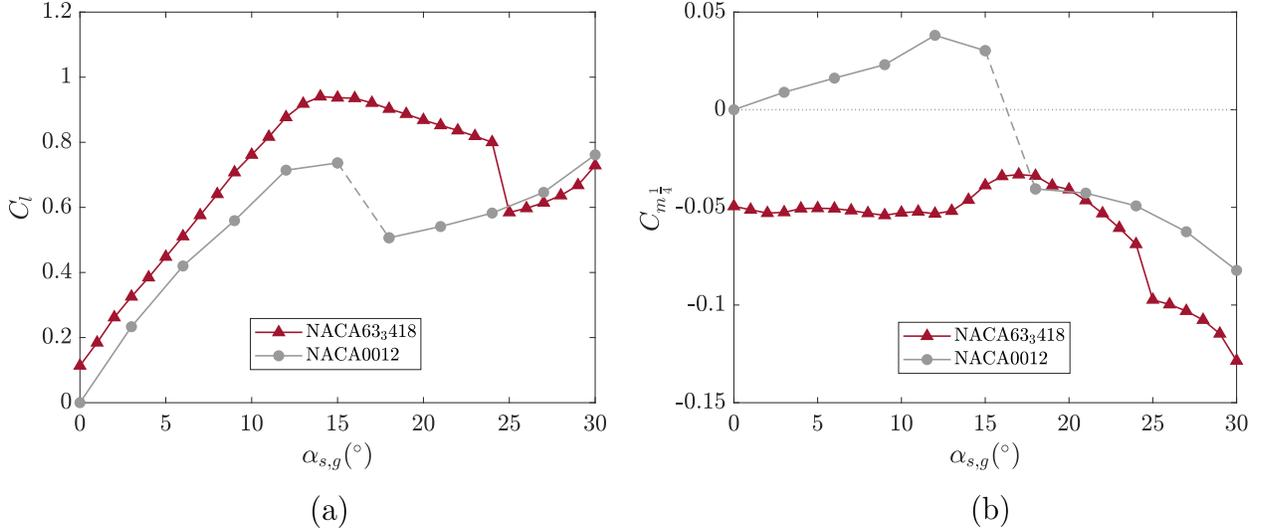
**Fig. 2 Comparison of the (a) lift coefficients and (b) pitching moment coefficients at the quarter chord between the two NACA airfoils. The angle resolution being too poor to measure precisely the static stall angle for the NACA0012 airfoil, dashed lines were chosen around the stall angle in order not to mislead the reader.**
