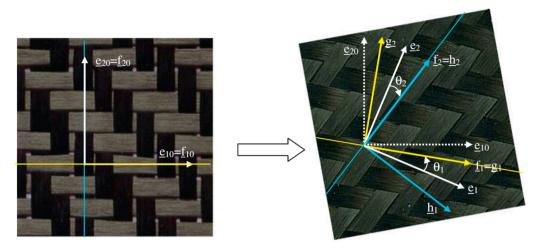
Fig. 3. Orthonormal frames in the fiber direction and the Green Naghdi frame. (For interpretation of the references to colour in this figure legend, the reader is referred to the web version of this article.)
