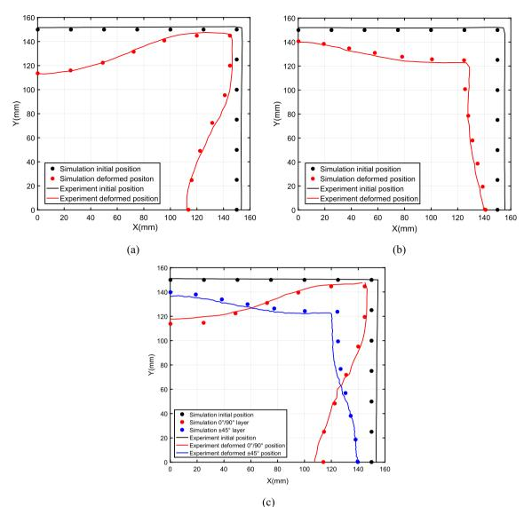
**Fig. 14.** Hemispherical forming fabric contour comparison between simulation and experiments. (a) Single layer of  $0^{\circ}/90^{\circ}$ . (b) Single layer of  $\pm 45^{\circ}$ . (c) Four-layer quasi-isotropic layup. (For interpretation of the references to colour in this figure legend, the reader is referred to the web version of this article.)
