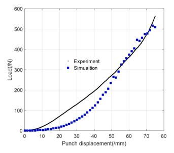
**Fig. 15.** Draping force during the hemispherical forming of a four-layer quasiisotropic stack. Comparison of experimental and numerical force. (For interpretation of the references to colour in this figure legend, the reader is referred to the web version of this article.)
