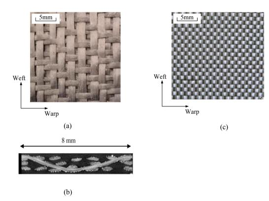
Fig. 4. (a) Interlock G1151 fabric. (b) X-ray Tomography of G1511 fabric [66]. (c) Plain weave fabric.
