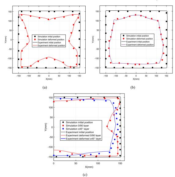
**Fig. 21.** Comparison of fabric profile from tetrahedral forming obtained by simulation and experiments. (a) Single layer of  $0^{\circ}/90^{\circ}$ . (b) Single layer of  $\pm 45^{\circ}$ . (c) Fourlayer quasi-isotropic layup. (For interpretation of the references to colour in this figure legend, the reader is referred to the web version of this article.)
