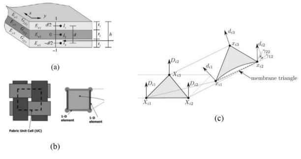
Fig. 2. Different approaches to decouple bending and tension stiffness. (a) The textile reinforcement is considered as a laminate [31]. (b) Modeling by beam and membrane element [37]. (c) Superposition of a membrane and shell element [43].
