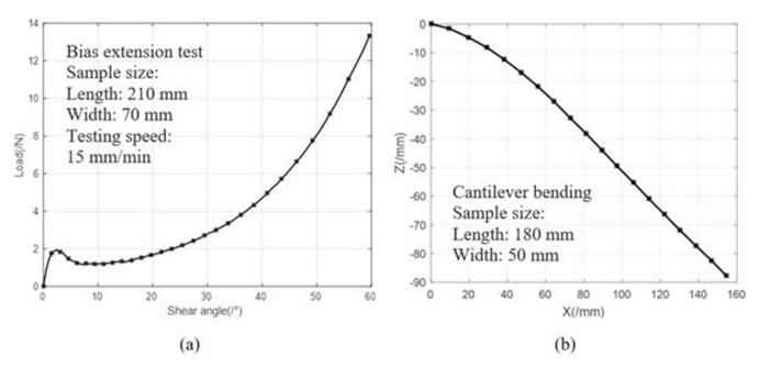
Fig. 9. Testing G1151 properties. (a) Bias extension test curve. (b) Cantilever bending curve. (For interpretation of the references to colour in this figure legend, the reader is referred to the web version of this article.)
