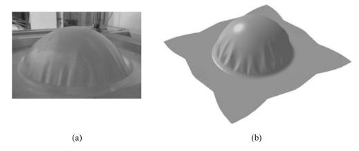
Fig. 16. Hemispherical forming of four layers quasi-isotropic plain weave. (a) Experiment result [90]. (b) Simulation result.
