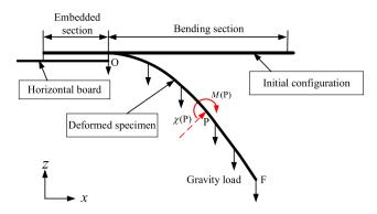
**Fig. 7.** Schematic diagram of bending test. (For interpretation of the references to colour in this figure legend, the reader is referred to the web version of this article.)
