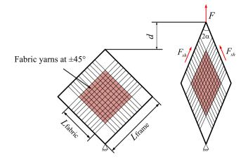
**Fig. 5.** Schematic diagram of picture frame test. (For interpretation of the references to colour in this figure legend, the reader is referred to the web version of this article.)
