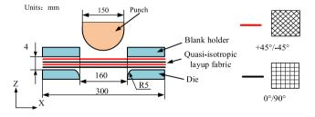
**Fig. 12.** Hemisphere forming geometry parameters. (For interpretation of the references to colour in this figure legend, the reader is referred to the web version of this article.)
