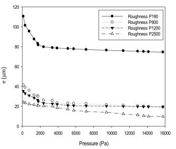
Fig. 9. Effect of pressure load on the liquid film thickness.
