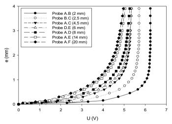
Fig. 6. Calibration curves for the different conductimetric probes.
