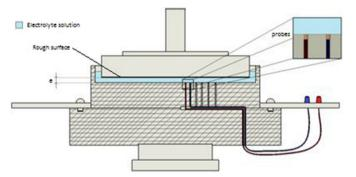
Fig. 3. Measurement test-section of liquid film thickness "e".
