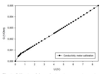
Fig. 5. Calibration of the conductimetric system using passive resistances at f = 50 kHz.
