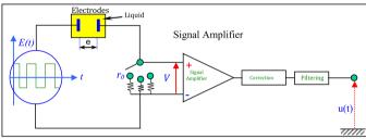
Fig. 4. Simplified sketch of the conductimetry measurement device.
