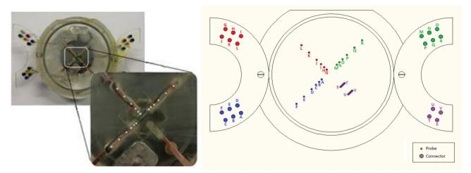
Fig. 2. Electrodes' arrangement in the bottom inert surface.
