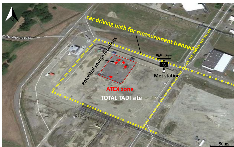
Figure 1. A schematic of the experimental setup on the top of the satellite image of the TADI platform (source: Google Earth © Google Earth). The red stars show some of the possible approximate location of the emission sources in the ATEX zone (rectangle with red colored line). The full set of exact locations used for the releases is detailed in Fig. S1 of the Supplement. A hybrid SUV drove in electric mode on the road next to the site, along the yellow colored double dotted lines. The meteorological station installed and operated by TOTAL was located at the basis of its black symbol.
