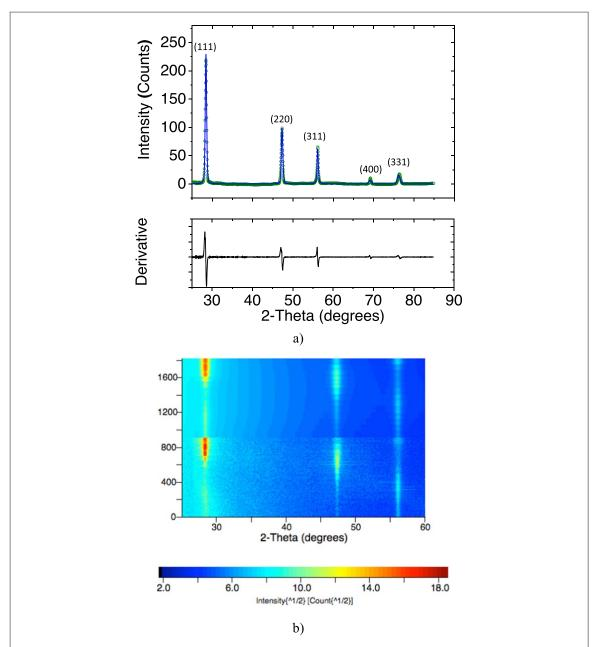
**Figure 4.** (a) Sum of the 936 diffraction diagrams of the sample and (b) 2D representation of all measured (bottom) and refined (top) diagrams showing the texture in the films (along the vertical axis are developed 936 experimental and 936 refined diagrams for as many  $(\chi, \varphi)$  orientations).
