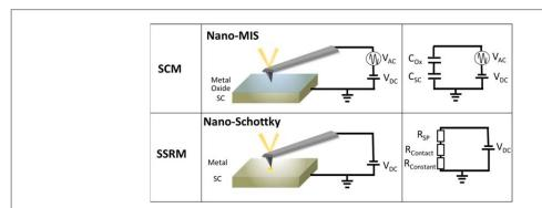
Figure 2. Nano-MIS and nano-Schottky of the SCM and SSRM modes, respectively, with their respective equivalent circuits.
