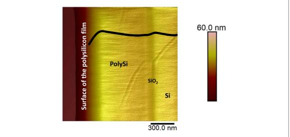
Figure 6. Surface topography  $(1.5~\mu\text{m} \times 1.5~\mu\text{m})$  of the cross-sectional sample. The profile of the surface is added in black.
