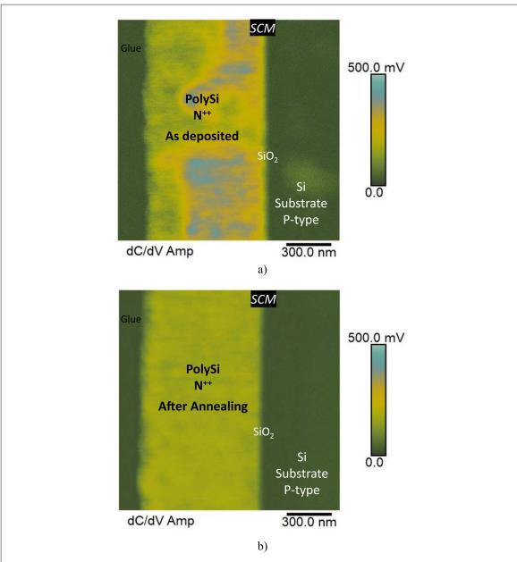
Figure 10. SCM maps  $(1.5 \,\mu\text{m} \times 1.5 \,\mu\text{m})$  on the cross sectionnal sample (a) for the as-deposited n<sup>++</sup> polysilicon layer and (b) after annealing.
