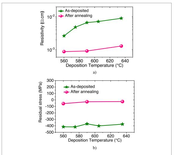
$\textbf{Figure 3.} \ Impact of the deposition temperature of \textit{in situ} doped \ LPCVD \ polysilicon \ layers (for 6 inch silicon \ wafers) \ before \ and \ after \ annealing: (a) layer resistivity \ and (b) \ residual \ stresses.$
