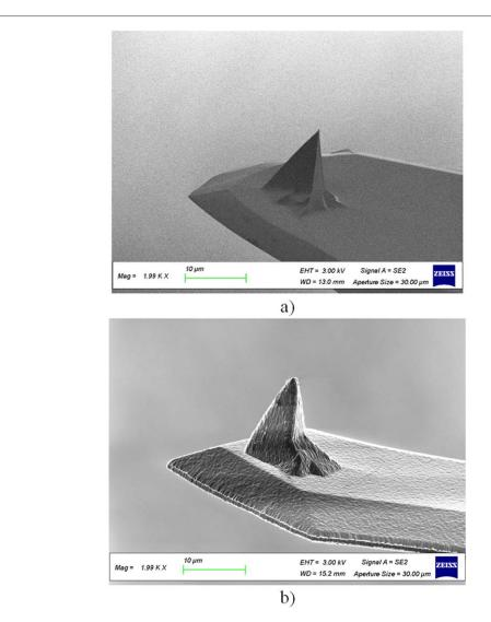
$\textbf{Figure 1.} \ S canning \ Electron \ Microscopy \ views \ of the used probes \ (a) \ Pt/Ir \ coated \ highly \ n-doped \ silicon \ probe \ SCM-PIC \ (b) \ highly \ conductive \ full \ diamond \ Adama \ tip \ (AD-40-AS) \ for \ SSRM \ measurements.$
