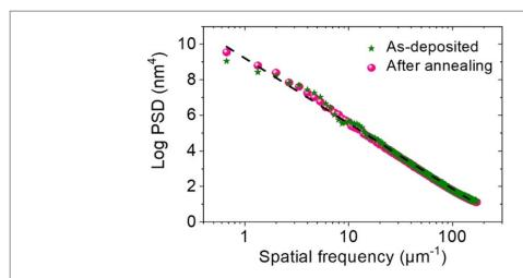
**Figure 7.** 2D Power spectral density (PSD) as a function of spatial frequency. for the AFM topography acquisitions (1.5  $\mu$ m  $\times$  1.5  $\mu$ m) of the as-deposited and annealed samples. The linear fitting (semi-logarithmic plot) is added in black.
