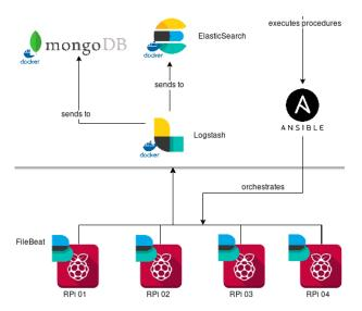
Fig. 1. Technical architecture for collecting Bluetooth signal.
