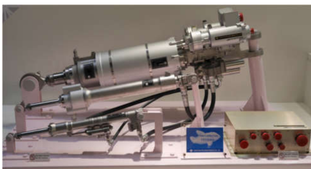
Figure 20. Mutualization of electrically supplied hydraulic generation for landing gears, Thermae II project.
