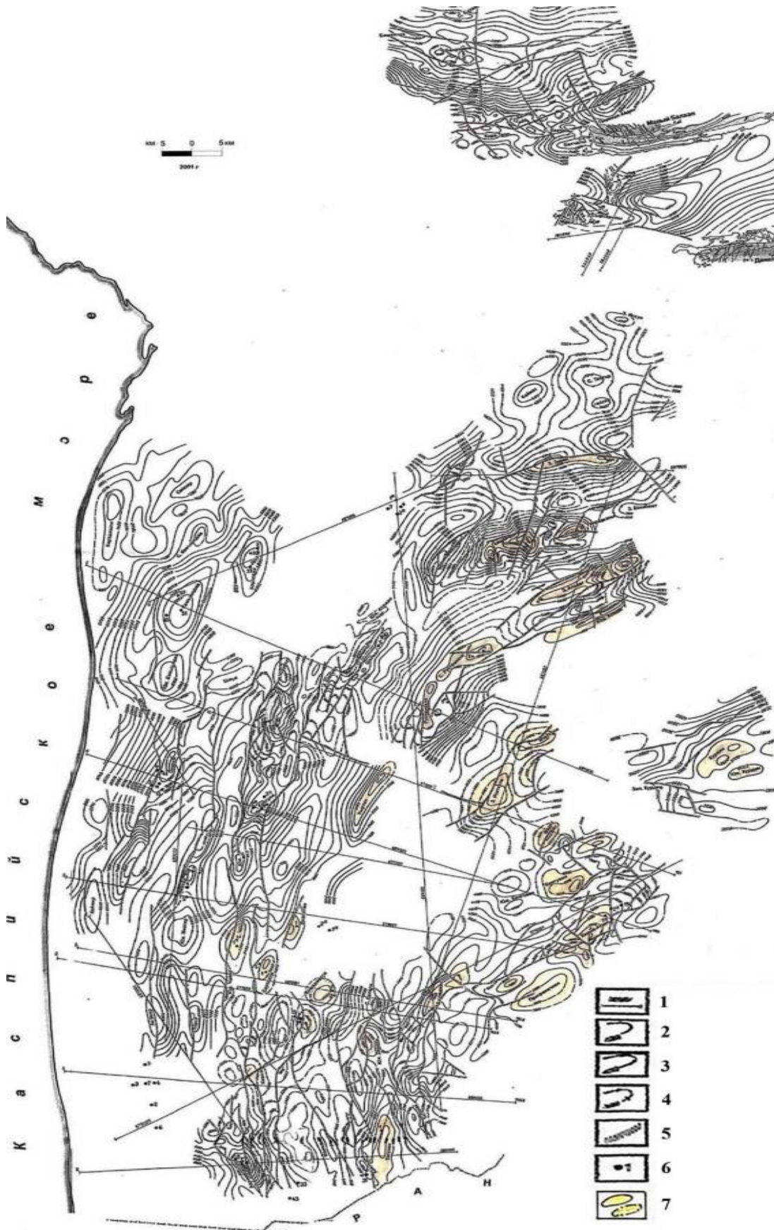
1 - common mid-point method profiles; 2 - contour lines of phantom seismic horizon mapped close to Neocomian bottom; 3 - contour lines of phantom seismic horizon mapped close to Neocomian top; 4 - contour lines of phantom seismic horizon mapped inside Lower Cretaceous deposits; 5 – tectonic faults from seismic survey data; 6 – deep drilling wells; 7 - the most accessible due to their depth anticline and anticline-block Malm-Neocomian objects recommended for preparation and exploration
