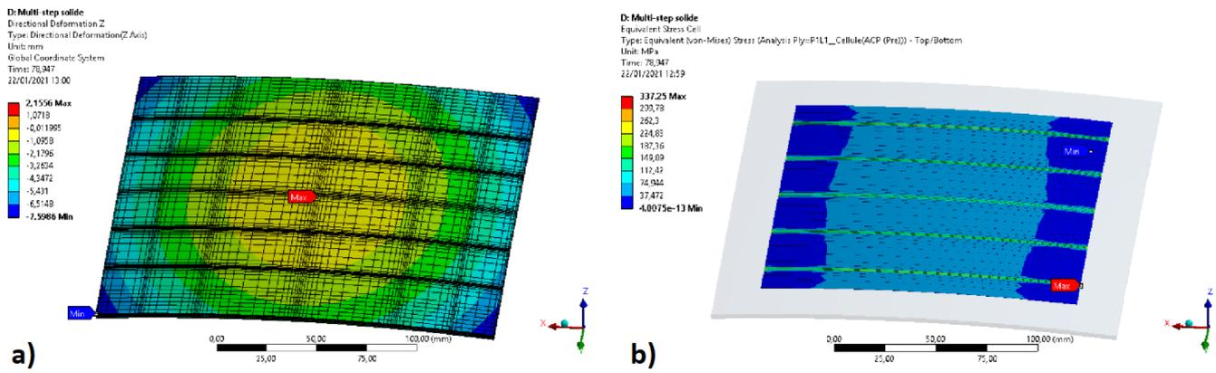
Figure 1: a) Z deformation and mesh for a double curved cell. b) Stresses in the cell resulting from the cooling in the mold.
