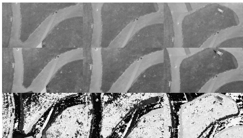
Figure 16: Excerpt of some images from the outdoor navigation. Desired virtual images appear at the top row, onboard images appear at the central row and images of difference appear at the bottom row.
