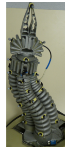
(a) Real soft continuum robot (b) Kinematics reconstruction Fig. 10: 3D CBHA Shape in free case
