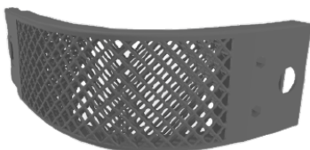
CAD Model of a curved grate from DIMOFAC project
