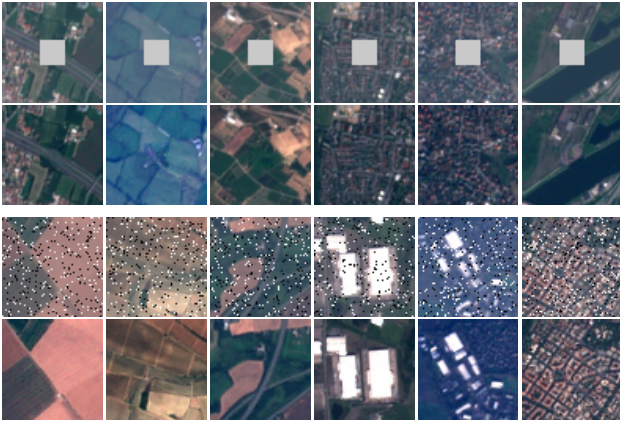
Figure 4: Image completion on EuroSAT dataset. Two up rows: inpainting, 12.5% information missing at the center. Two bottom rows: pixel defect correction, 10% salt and pepper noise.
