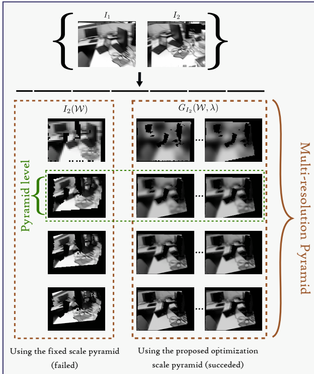
Figure 1: The considered algorithms aim at aligning the image pair \{I_1, I_2\} , where the images resulting from the alignment are G_{I_2}(\mathcal{W}, \lambda) and I_2(\mathcal{W}) . Here the fixed scale pyramid-based method was unable to align the image pair because it fell in a local minimum, while the proposed optimized scale pyramid-based method succeeded because it is able to automatically adapt the image smoothing to suppress local minima.
