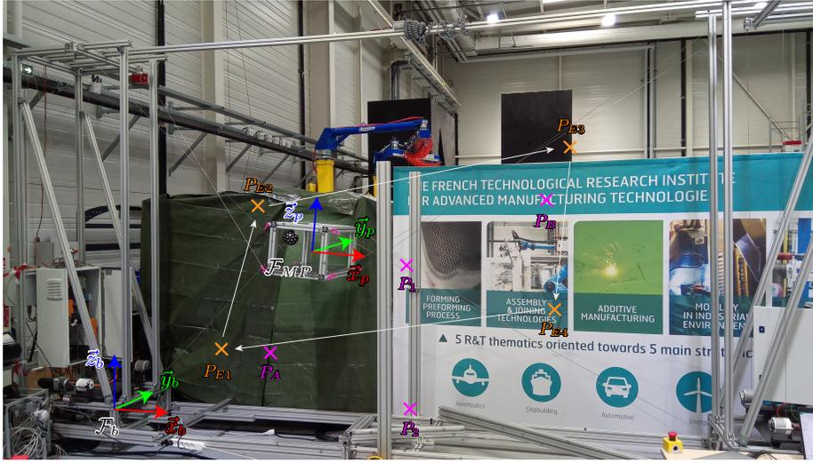
Fig. 2: Test path, targets and MP home poses
