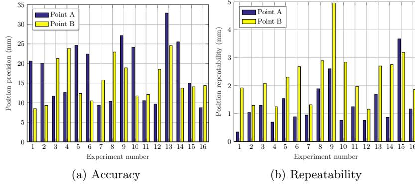
Fig. 6: Position accuracy and repeatability for each experiment
