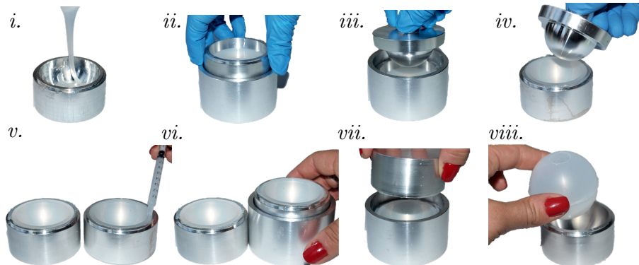
FIG. 8. Shell fabrication process. i. Mixed and degassed DragonSkin 30 is poured into two hemispherical aluminum cavities of R_o = 25 mm. Only one is shown in i.-iv. , and several layers of tape have been cut into a circle and adhered to the center of one of the hollow spheres. ii. After degassing again, the filled cavity is fitted with an alignment sleeve. iii. A half-sphere of R_i < R_o is inserted. iv. After curing for 25 minutes in the oven, a spherical hemisphere has formed. v. Heptane-diluted polymer is deposited with a syringe to glue two cured hemispheres. vi.-vii. The edges of the two hemispheres are joined and aligned by the alignment sleeve. viii. After curing at room temperature for at least 16 hours, a sealed sphere is removed from the mold.
