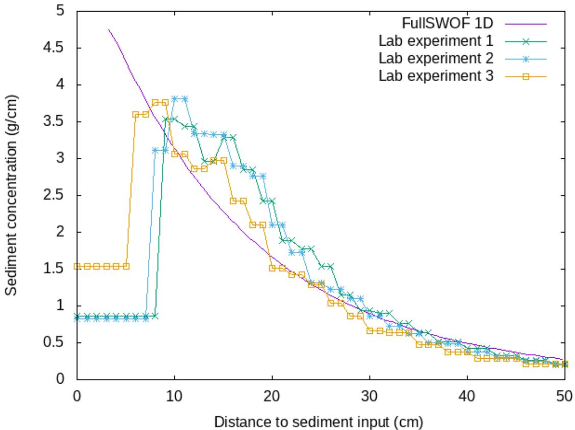
**Figure 2:** Sediment deposit on the domain at the end of the experimental runs, and for a 1-to-9 ratio of sediment velocities equal to 5 and 16 mm s<sup>-1</sup>, respectively, with a 3 cm shift.
