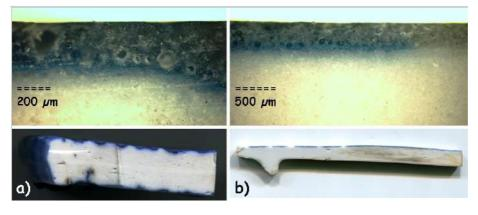
Fig. 3. Representative shards and their sections of blue-andwhite Chinese porcelains: a) Qianlong (1736-1796) and b) Surcouf' shipwreck cargo (17th c.)
