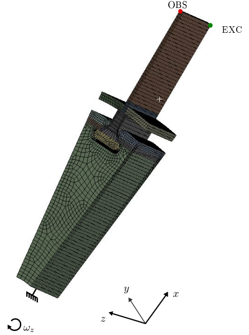
Figure 2: Sector of the studied model with boundary conditions.
