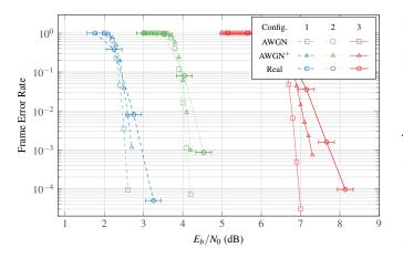
Fig. 4. DVB-S2 FER decoding performance.
