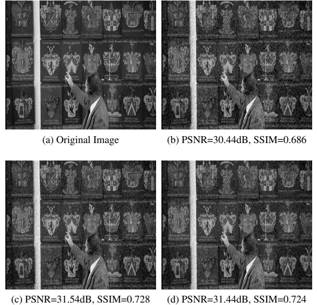
Fig. 6: Visual quality comparison at a CSNR = 0dB and full available bandwidth for Shields sequence (first frame). From left to right, top to down: (a) Original image, (b) Classic SoftCast, (c) OPA-SoftCast, (d) The proposed method.
