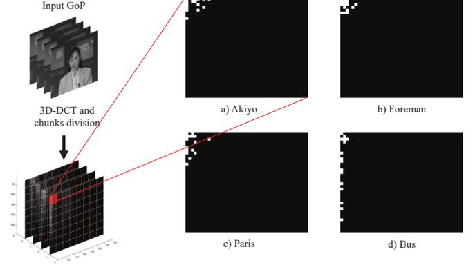
**Fig. 3:** Visual representation of the position of the 16 selected SFC (small white squares) by OPA-SoftCast in the upper left chunk ( $44 \times 36$  coefficients) of the first frame of the GoP for the selected CIF video sequences.
