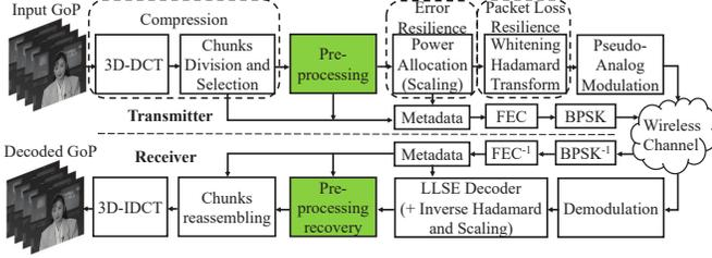
Fig. 1: Block diagram of the *SoftCast* scheme.
