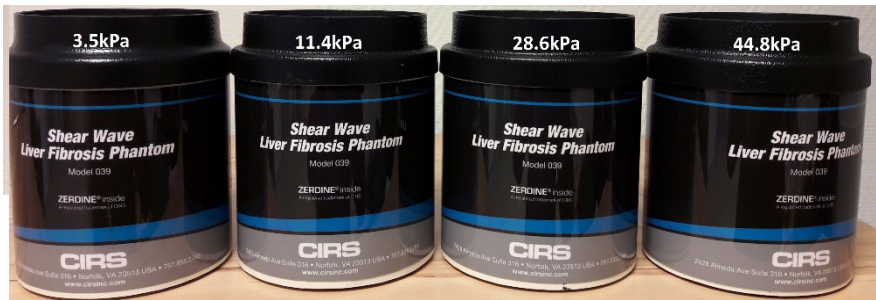
Figure 1: Set of CIRS test phantoms {C1, C2, C3, C4} calibrated for liver fibrosis at 3.5, 11.4, 28.6 and 44.8 kPa
