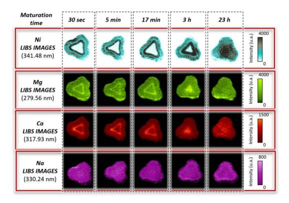
Figure 2. Ni, Mg, Ca, and Na LIBS intensities images for varying maturation times  $T_M$  for [CA]=0.2 mol/L.
