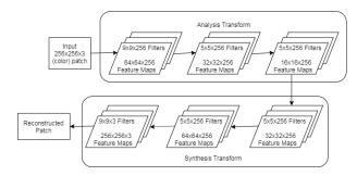
Fig. 2. Architecture of CNN used as feature extractor.
