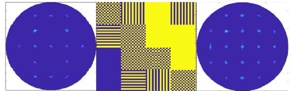
Fig. 6. Example of input and corresponding output to the algorithm: wanted radiation pattern with  $\phi=135^\circ$  (1<sup>st</sup> image); obtained coding matrix in output (2<sup>nd</sup> image) and radiation pattern corresponding to that coding matrix (3<sup>rd</sup> image).
