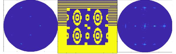
Fig. 5. Example of input and corresponding output to the algorithm: wanted radiation pattern with  $\phi=0^\circ$  (1<sup>st</sup> image); obtained coding matrix in output (2<sup>nd</sup> image) and radiation pattern corresponding to that coding matrix (3<sup>rd</sup> image).
