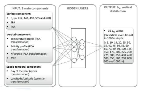
Fig. 1. Schematic overview of the SOCA2020 multi-layer perceptron that retrieves the vertical distribution of bbp from merged satellite and Argo data associated with the longitude/latitude/day of the year of the considered satellite-to-Argo matchup.
