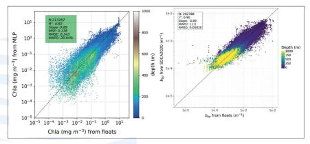
Fig. 3. Comparison of the Chl values retrieved by SOCA2020 to the reference measurements acquired by: a) BGC-Argo profiling floats from the independent validation dataset (left panel) and b) HPLC from MAREDAT database and LOV-IMEV database (right panel)
