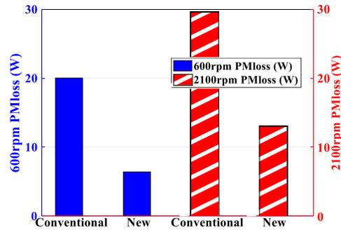
Fig. 8. PM loss at 600 and 2100 r/min.
