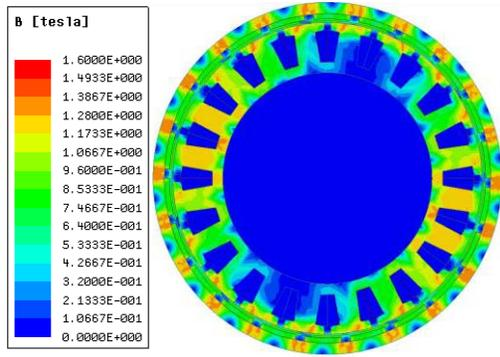
Fig. 5. Flux density of two machines under un-load.
