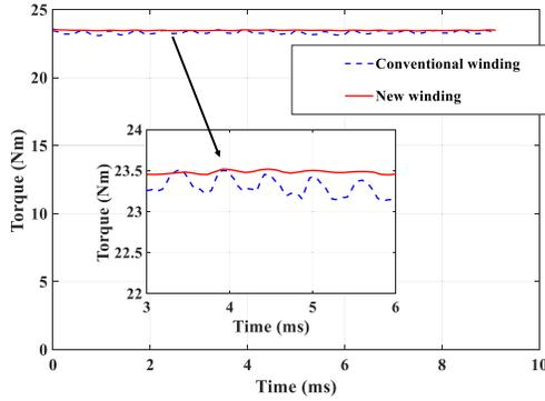
Fig. 10. Comparison of electromagnetic torque.
