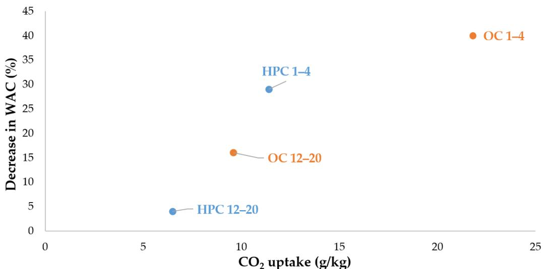
Figure 15. Relationship between the decrease of the WAC and the CO<sub>2</sub> uptake of RCAs obtained from laboratory concretes.
