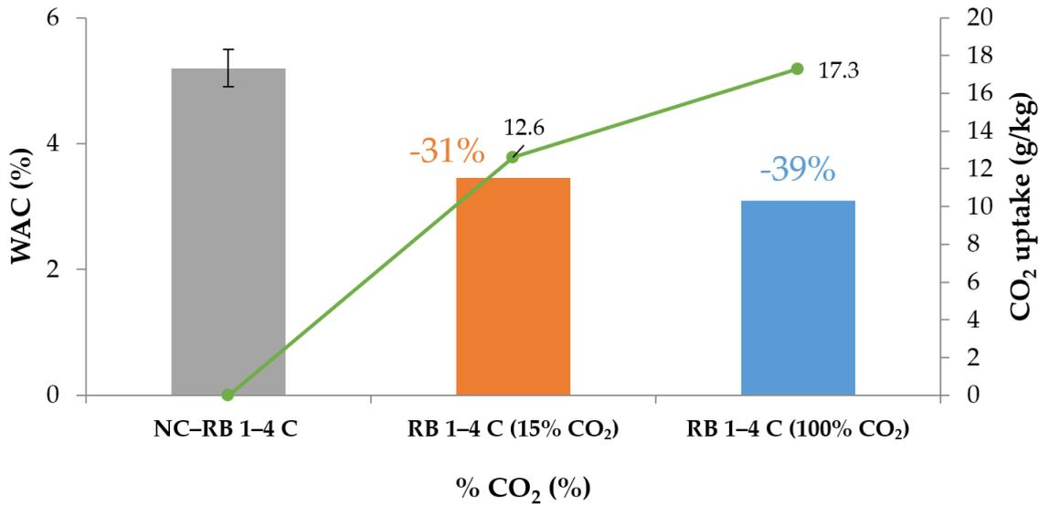
Figure 17. Effect of the CO<sub>2</sub> concentration on the CO<sub>2</sub> uptake and WAC (one WAC measurement for RCAs after carbonation).
