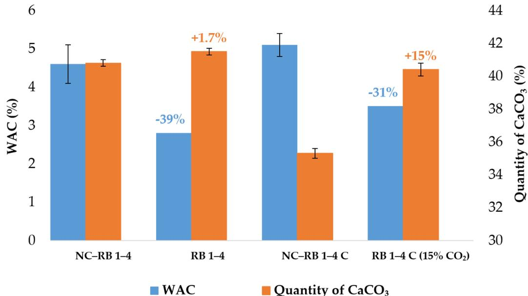
**Figure 16.** Correlation between the WAC and the formation of CaCO<sub>3</sub> (one WAC measurement for RCAs after carbonation).
