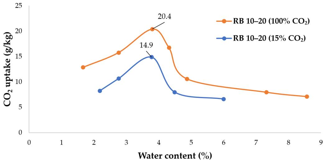
**Figure 6.** Effect of the CO<sub>2</sub> concentration on CO<sub>2</sub> uptake as a function of the water content (one accelerated carbonation test for these RCAs at the same water content).
