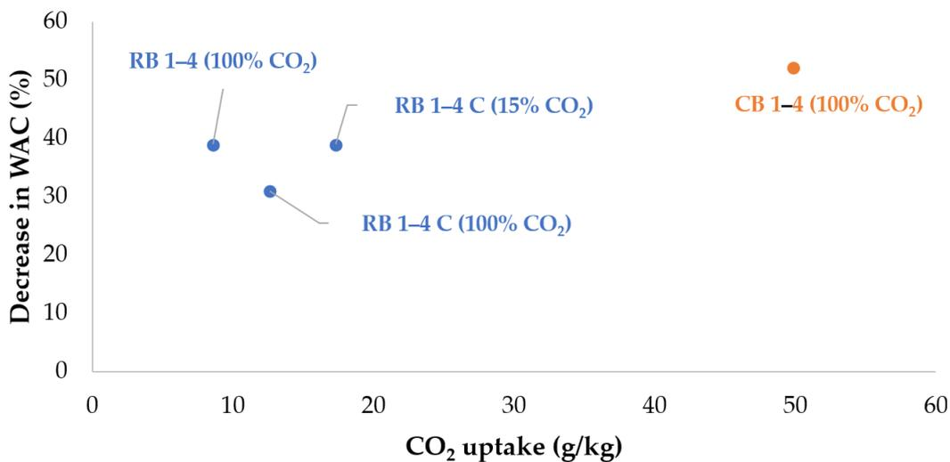
Figure 14. Relationship between the decrease in the WAC and the CO<sub>2</sub> uptake of RCAs sourced from demolition concretes.
