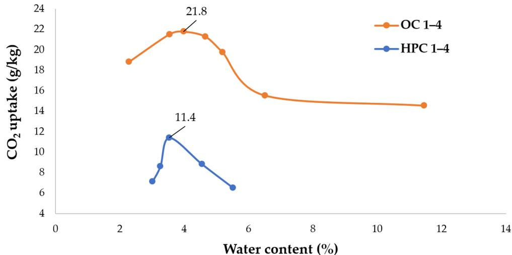
**Figure 8.** Effect of the RCA type on CO<sub>2</sub> uptake as a function of the water content (one accelerated carbonation test for these RCAs at these water contents).
