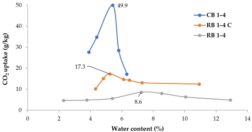
Figure 4. Effect of the initial natural carbonation of an RCA on CO<sub>2</sub> uptake as a function of the water content (one accelerated carbonation test for these RCAs at these water contents).
