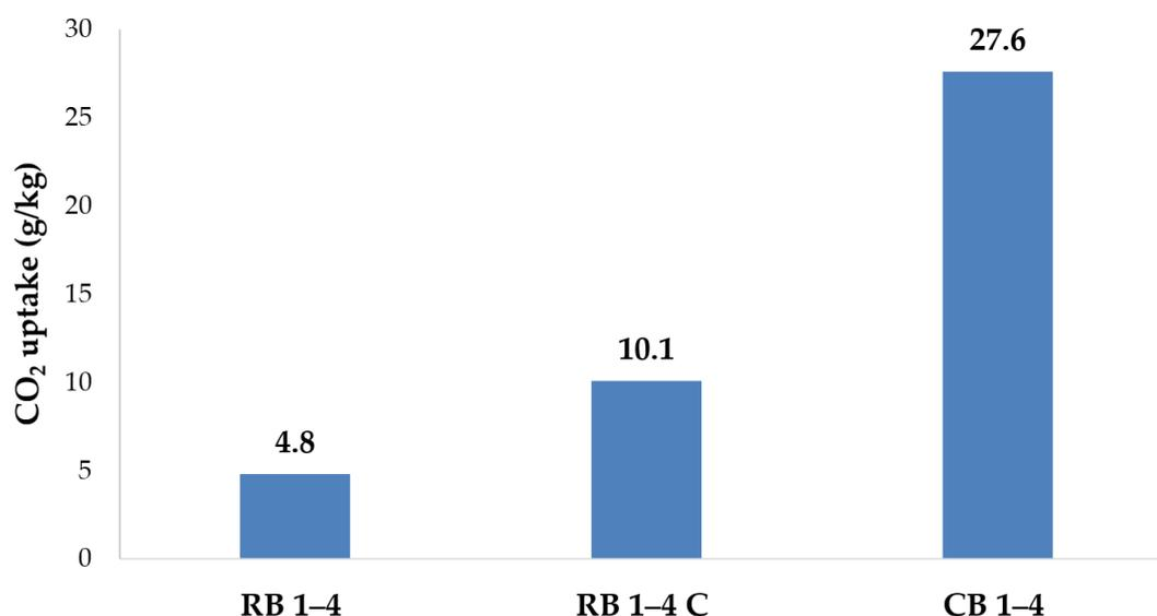
**Figure 5.** Rate of CO<sub>2</sub> uptake for each RCA with the same water content (4%) (one accelerated carbonation test for these RCAs at the same water content).
