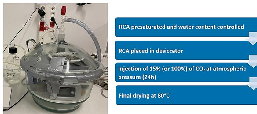
**Figure 1.** Experimental setup for the accelerated carbonation test.
