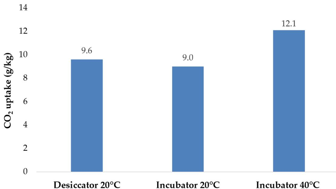
**Figure 10.** Effect of the temperature on CO<sub>2</sub> uptake (water content of 2.8%) (one accelerated carbonation test for these RCAs at this same water content).
