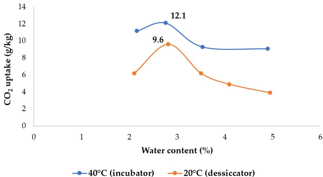
**Figure 11.** Effect of the water content on the CO<sub>2</sub> uptake (at 20 °C and 40 °C) for OC 12–20 (one accelerated carbonation test for these RCAs at these water contents).
