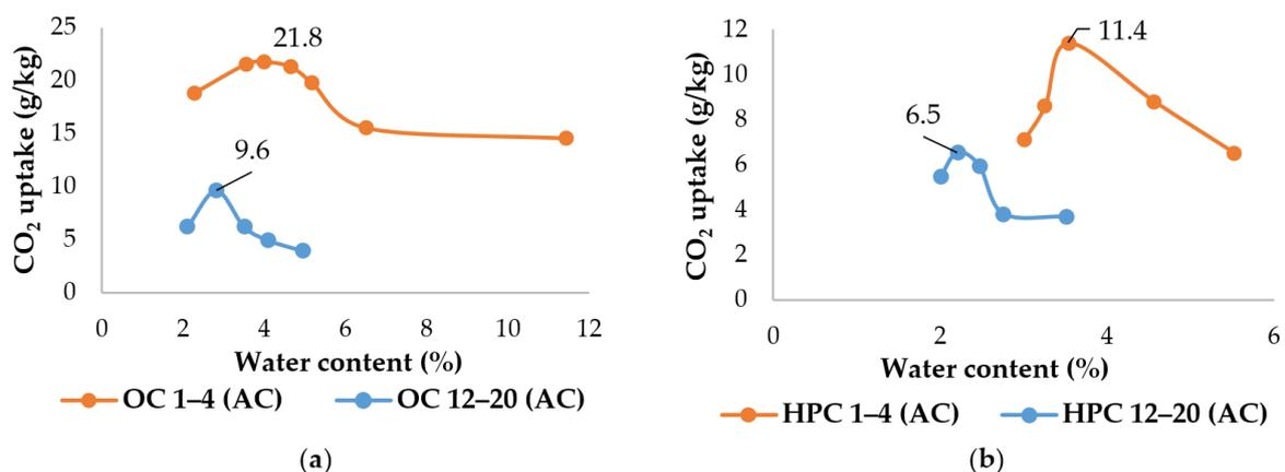
**Figure 9.** Effect of the RCA size on the CO<sub>2</sub> uptake (a) for OC and (b) for HPC (one accelerated carbonation test for these RCAs at these water contents).
