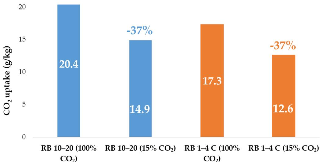
**Figure 7.** Effect of the CO<sub>2</sub> concentration on the CO<sub>2</sub> uptake (RB 10–20 and RB 1–4 C) (one accelerated carbonation test for these RCAs at these water contents).
