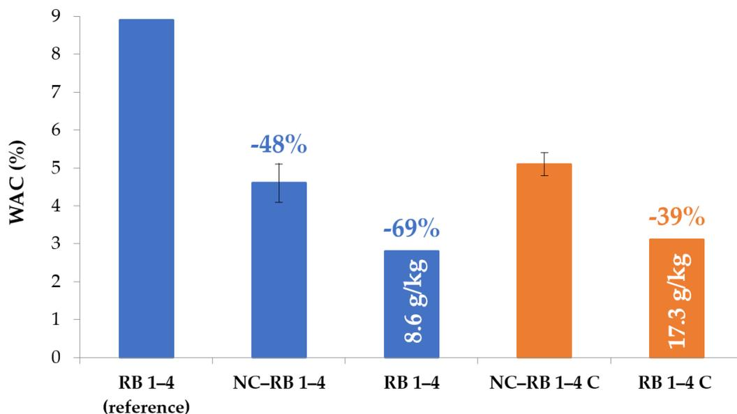
**Figure 13.** Effect of carbonation (natural and accelerated) on the WAC (one WAC measurement for each RCA after carbonation).
