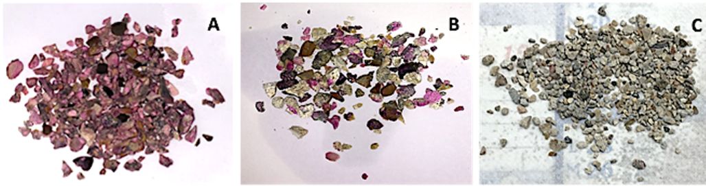
Figure 3. Phenolphthalein spray on RCA (A) CB 1–4, (B) RB 1–4 C and (C) RB 1–4.
