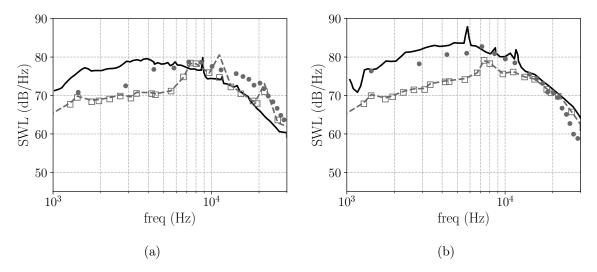
Figure A.2: Comparison of the SWL of the original Ventres model and the Ventres model with the 2D Posson response using the anisotropic spectrum of Nallasamy and Envia [36]. Experiment (—), Nallasamy and Envia's result ( • ), Ventres - 500 pts (---), Posson 2D ( □ ). (a) Upstream SWL, (b) Downstream SWL.
