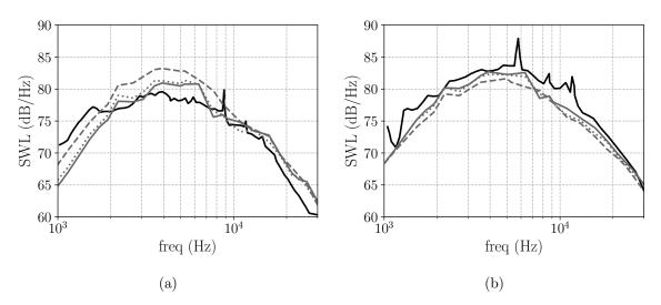
Figure 12: Stagger angle effect, Posson's model. Experiment (—),  $\chi_{geo}$  (—),  $\chi_{A50B50}$  (·····),  $\chi_{A90B10}$  (---). (a) Upstream SWL, (b) Downstream SWL.
