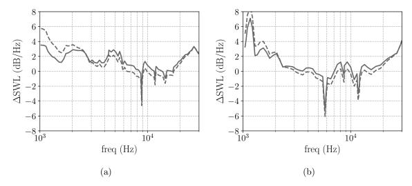
Figure 20: Predictions using Hanson's model with both Liepmann's and von Kármán's spectra. SWL difference with respect to the noise measurements. Liepmann's spectrum (——), von Kármán's spectrum (---). (a) Upstream ΔSWL, (b) Downstream ΔSWL.
