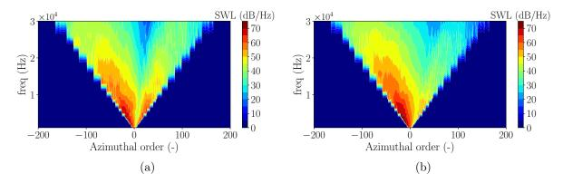
Figure 15: Upstream modal amplitude for different stagger angles, Posson's model. (a)  $\chi_{A50B50}$ , (b)  $\chi_{A90B10}$ .
