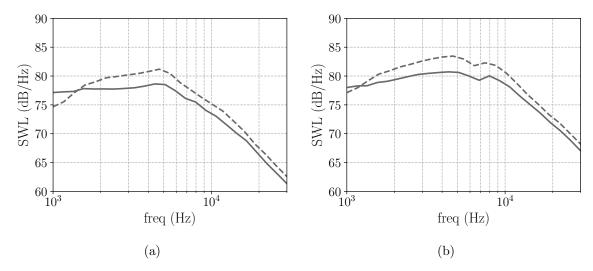
Figure 17: Mean flow variation effect, Hanson's model. Nallasamy and Envia's RANS (——), Leonard *et al.*'s RANS (——-). (a) Upstream SWL, (b) Downstream SWL.
