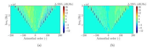
Figure 28: Modal amplitude difference between Posson's and Amiet's models, baseline configuration with 27 vanes. (a) Upstream  $\Delta$ SWL, (b) Downstream  $\Delta$ SWL.
