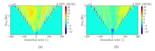
Figure 27: Modal amplitude difference between Posson's and Amiet's models. (a) Upstream  $\Delta$ SWL, (b) Downstream  $\Delta$ SWL.
