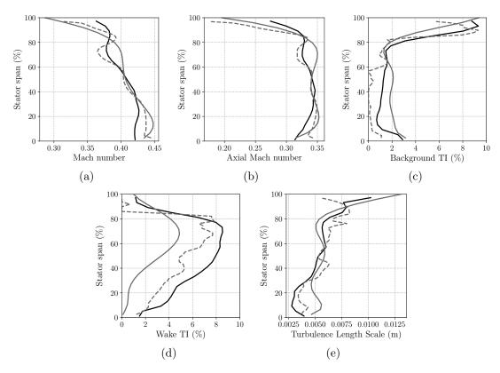
Figure 9: Comparison of the model input parameter extractions performed on two different RANS simulations. Experiment (—), Nallasamy and Envia's RANS (—), Leonard *et al.*'s RANS (---). (a) Mach number, (b) Axial Mach number, (c) Background turbulence intensity, (d) Wake turbulence intensity, (e) Turbulence length scale.
