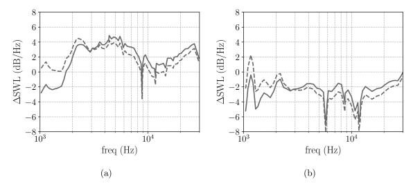
Figure 21: Predictions using Posson's model with both Liepmann's and von Kármán's spectra. SWL difference with respect to the noise measurements. Liepmann's spectrum (——), von Kármán's spectrum (——-). (a) Upstream ΔSWL, (b) Downstream ΔSWL.
