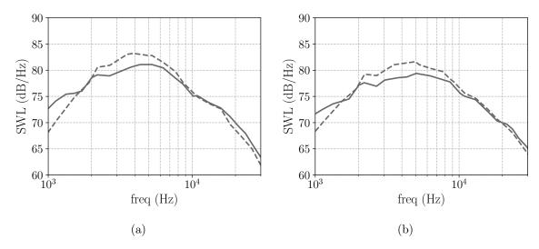
Figure 18: Mean flow variation effect, Posson's model. Nallasamy and Envia's RANS (——), Leonard *et al.*'s RANS (——-). (a) Upstream SWL, (b) Downstream SWL.
