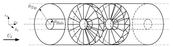
Figure 3: Fan stage configuration for the acoustic models.
