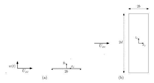
Figure 4: Amiet's model configuration. (a) Unwrapped strip, (b) 3D view of an isolated vane with the corresponding impinging flow.
