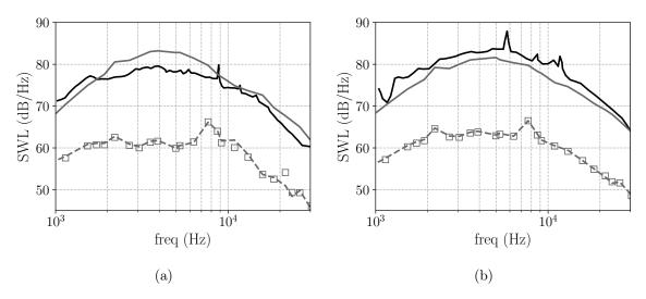
Figure 19: Comparison of the SWL of 2D and 3D models with Liepmann's spectrum (2D or 3D). Experiment (—), Posson (—), Ventres (---), Posson 2D (□). (a) Upstream SWL, (b) Downstream SWL.
