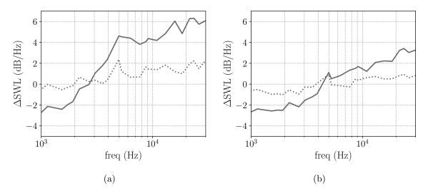
Figure 26: Cascade effect. SWL difference between Posson's model and Amiet's model predictions. Baseline configuration with 54 vanes (—), Reduced configuration with 27 vanes (·····). (a) Upstream  $\Delta$ SWL, (b) Downstream  $\Delta$ SWL.
