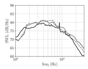
Figure 13: Stagger angle effect, Masson's model. Experiment (—),  $\chi_{geo}$  (—),  $\chi_{A50B50}$  (·····),  $\chi_{A90B10}$  (= - -). Upstream SWL.
