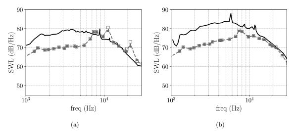
Figure A.1: Comparison of the SWL of the original Ventres model for different number of discretization points using the anisotropic spectrum of Nallasamy and Envia [36]. Experiment (—), 300 pts (  $\bullet$  ), 400 pts ( - -  $\cdot$ ), 500 pts (  $\Box$  ). (a) Upstream SWL, (b) Downstream SWL.
