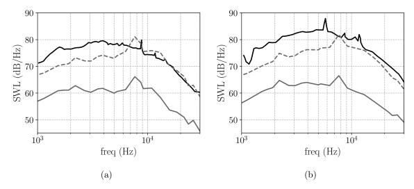
Figure 22: Predictions using Ventres' model with both Liepmann's and Nallasamy and Envia's spectra. Experiment (—), Liepmann's spectrum (—), Nallasamy and Envia's spectrum (—-). (a) Upstream SWL, (b) Downstream SWL.
