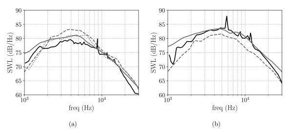
Figure 29: Propagation effect. Experiment (—), Hanson (—), Posson (---), Masson (·····). (a) Upstream SWL, (b) Downstream SWL.
