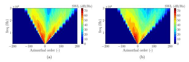
Figure 14: Upstream modal amplitude for different stagger angles, Masson's model. (a)  $\chi_{A50B50}$ , (b)  $\chi_{A90B10}$ .
