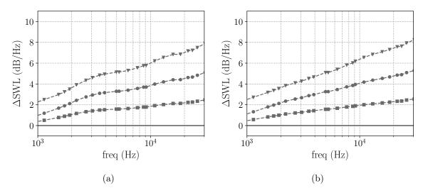
Figure 23: Predictions using Posson's model with Kerschen and Gliebe's spectrum  $(l_a/l_t < 1)$ . SWL difference with respect to the isotropic case  $(l_a = l_t)$ .  $l_a = l_t$  (---),  $l_a = 0.9l_t$  (---),  $l_a = 0.8l_t$  (---),  $l_a = 0.7l_t$  (---). (a) Upstream  $\Delta$ SWL, (b) Downstream  $\Delta$ SWL.
