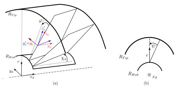
Figure 7: Introduction of the sweep angle  $\varphi$  and the lean angle  $\psi$  as proposed by Hanson.  $(x'_c, y'_c, z'_c)$  is the reference frame before the sweep angle rotation, which leads to the reference frame  $(x_c, y_c, z_c)$ . (a) 3D view, (b) Front view.
