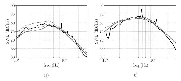
Figure 11: Stagger angle effect, Hanson's model. Experiment (—),  $\chi_{geo}$  (—),  $\chi_{A50B50}$  (·····),  $\chi_{A90B10}$  (= - -). (a) Upstream SWL, (b) Downstream SWL.
