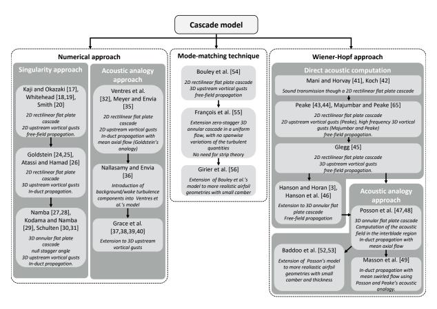
Figure 2: Classification of cascade models.
