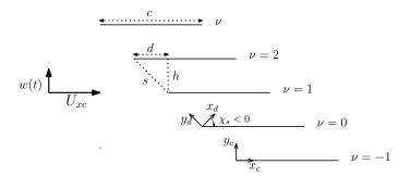
Figure 5: Unwrapped strip for the model of Ventres.
