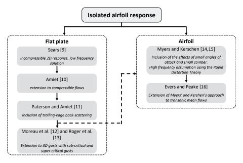
Figure 1: Classification of isolated airfoil models.
