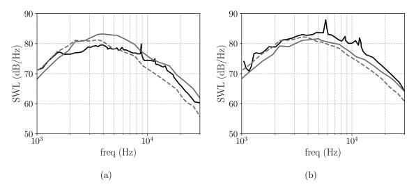
Figure 25: Cascade effect, baseline configuration. Experiment (—), Posson (—), Amiet 3D (---). (a) Upstream SWL, (b) Downstream SWL.
