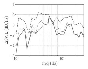
Figure 16: SWL difference between Posson and Masson's models for different stagger angle values.  $\chi_{geo}$  (—),  $\chi_{A50B50}$  (·····),  $\chi_{A90B10}$  (---). Upstream  $\Delta$ SWL.
