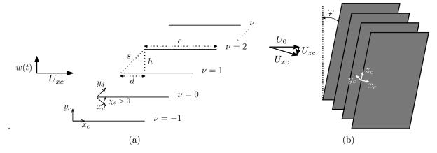
Figure 6: Glegg's model configuration. (a) Unwrapped strip, (b) 3D view of a vane cascade with a sweep angle  $\varphi$  and the corresponding impinging flow.
