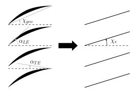
Figure 10: Equivalent flat plate geometry.
