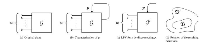
FIGURE 1 The concept of LPV modeling.
