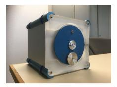
FIGURE 3 Unbalanced disc system: DC motor connected to a disc with added weight. The overall system functions as a rotational pendulum.
