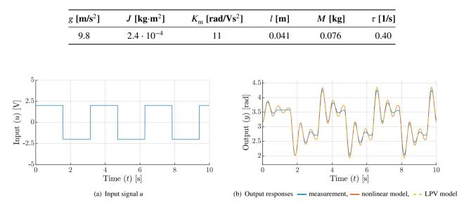
**TABLE 2** Identified parameters of the unbalanced disc system.
