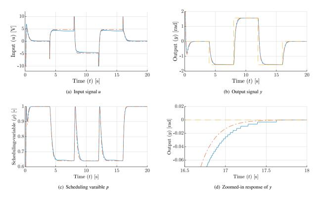
FIGURE 6 Closed-loop response with the LPV controller: -- experiment, -- simulation, -- reference.
