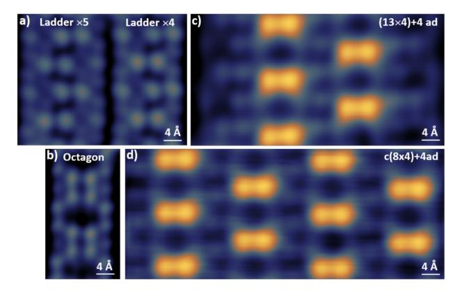
**Figure 2.** High-resolution STM images of adatom free motifs: (a) Ladder ×5 and Ladder ×4 motifs (I = 100 pA,  $V_{sample} = 100 \text{ mV}$ ), (b) Octagon motif (I = 5 nA,  $V_{sample} = 200 \text{ mV}$ ). High-resolution STM images of adatom-covered structures: (c) (13×4)+4adatoms structure (I = 460 pA,  $V_{sample} = -570 \text{ mV}$ ), (d) c(8×4)+4adatoms structure (I = 460 pA,  $V_{sample} = -570 \text{ mV}$ ). The STM images were acquired at 77 K in (a), (c), (d) and at RT in (b).
