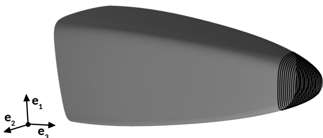
Figure 3: Needle tip given by level set \varphi = 0.5 ( \Omega = 0.30 and \varepsilon_0 = 3\% at t = 9 s). Intersections by transverse planes plotted at z \in [1; 19] .
