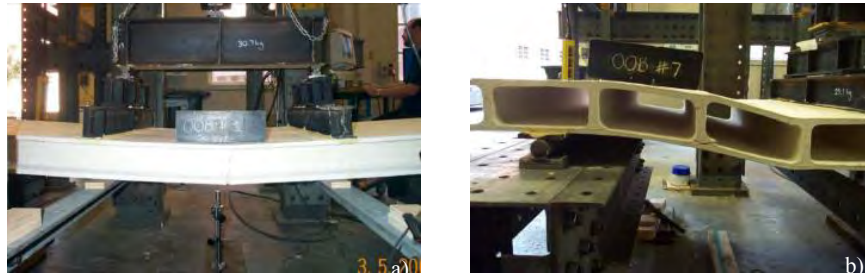
Fig. 3 Failure modes for out-of-plane bending of the panel: a) Ribs parallel to the span, b) Ribs perpendicular to the span [9]
