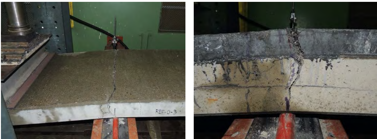
Fig. 8 Cracks at the top surface of the panels after executing experiments. Left figure is reference panel and right figure is detail of the panel with 30 mm UHPC.
