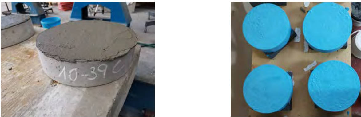
Fig. 8 Newly developed PRC; on the left: its application on the C8/10 underlying concrete, on the right: special impermeable sealant applied on other sides.
