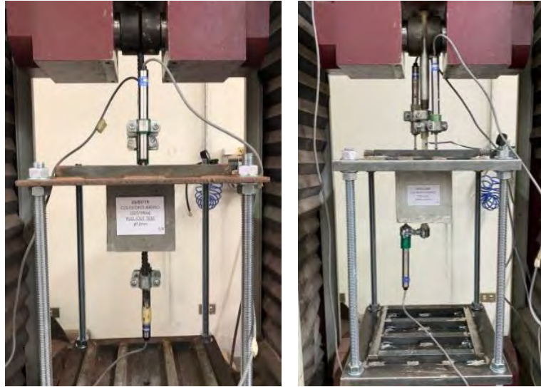
Fig. 2 Pull-out test setup of specimens with a) deformed steel bar; b) GFRP bar
