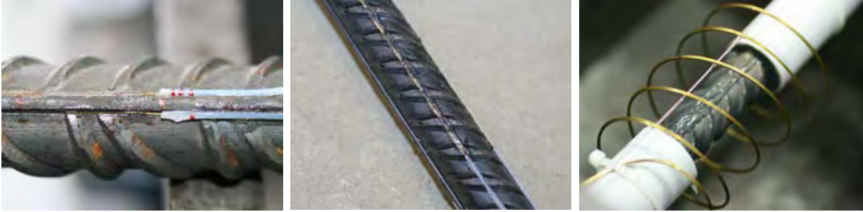
Fig. 6 Applied sensor fibre and protective tube; left: at the longitudinal rib; middle: in groove through the inclined ribs; right: with support frame in helix form.
