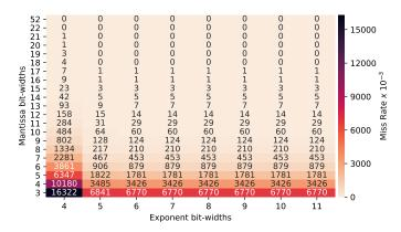
Figure 2: QoR variation as a function of the exponent  $E_d$  and mantissa  $M_d$  bit-widths.
