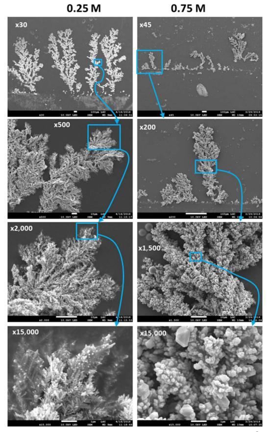
Figure 12. SEM images of copper branches, for two concentrations  $c_0$  of 0.25 and 0.75 M, and for a current density j of 66 mA cm<sup>-2</sup>.
