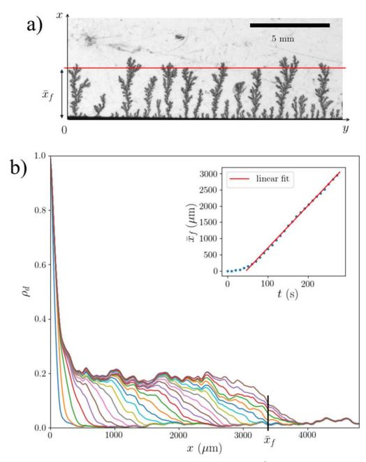
**Figure 6.** (a) Optical image of a ramified copper deposit obtained with  $c_0 = 0.5$  M, j = 266 mA cm<sup>-2</sup> after an electrolysis duration of 280 s, the red line indicates the average front location  $\bar{x}_f$  detected from the inflection point of the last S-shaped density profile shown in (b). (b) The corresponding density profiles  $\rho_d$  at several times (10 s between each curve), the insert shows the temporal evolution of  $\bar{x}_f$ .
