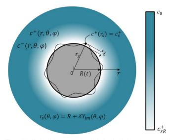
**Figure 14.** Sketch of the growth of a spherical grain (dark grey), surrounded by an electrically neutral and diffusional region (color map), and subject to shape deformations whose the amplitude is measured by  $\delta(t)$ .
