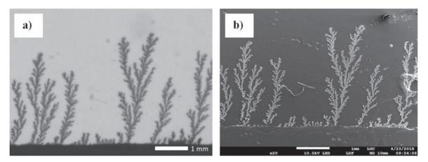
Figure 3. (a) Optical image of ramified copper branches taken during a galvanostatic electrolysis in the Hele-Shaw cell (elapsed time = 220 s,  $c_0 = 0.5$  M, j = 133 mA cm<sup>-2</sup> and non-metallized cell wall), (b) SEM image taken after the recovery of the deposit.
