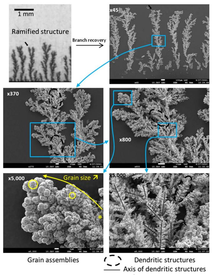
**Figure 9.** SEM images of a copper branch obtained for an applied current density of 266 mA cm<sup>-2</sup> and  $c_0 = 0.5$  M. One region is visualized by successively increasing the magnification. In order to focus on the main result, only some dendritic structures are indicated per image by black dashed line ellipses. The growth directions of the dendritic structures are indicated by gray lines.
