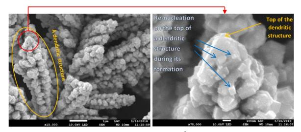
Figure 10. SEM images of a copper branch (central part) obtained with 0.5 M and 133 mA cm $^{-2}$ . This shows that the re-nucleation process is still present during the formation of copper dendritic structures.
