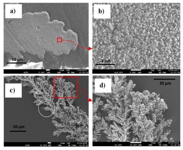
Figure 4. SEM images of copper branches obtained with gold metallization of cell walls, at a magnification of  $\times$ 550 in a) and  $\times$ 14000 in (b), and without metallization (with cell walls made of bare parafilm), at magnification of  $\times$ 450 in (c) and  $\times$ 15000 in (d); j = 133 mA cm<sup>-2</sup> and  $c_0 = 0.5$  M.
