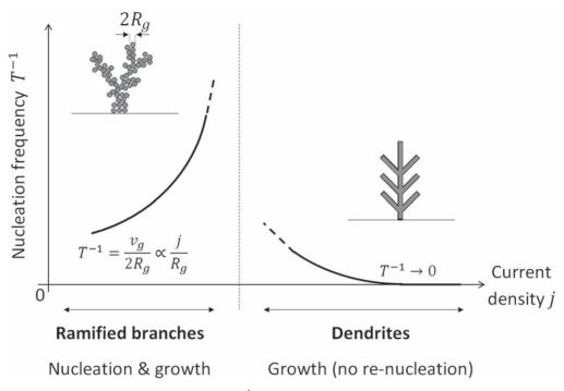
Figure 1. Illustration of the dependence of the nucleation frequency  $T^{-1}$  on the applied current density *j*, when the growth regime changes from re-nucleation process (ramified branches) to pure growth without re-nucleation process (dendrites).
