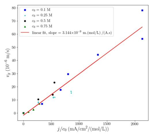
Figure 7. The average growth velocity  $v_g$  as a function of the ratio  $j/c_0$  for all of the investigated concentrations; the red line corresponds to the linear fit of all the points (the slope =  $3.144 \times 10^{-9}$  m.(mol l<sup>-1</sup>) (A.s)<sup>-1</sup>).
