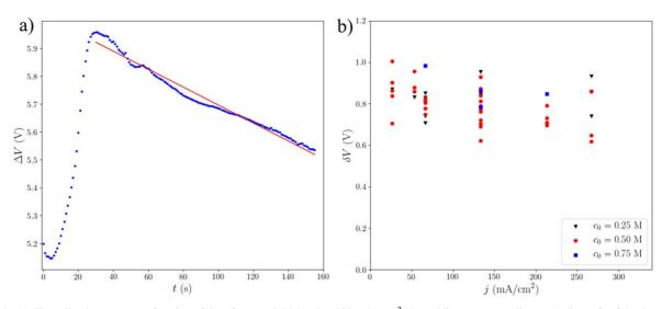
**Figure B-1.** (a) The cell voltage  $\Delta V$  as a function of time for  $c_0 = 0.5$  M and = 133 mA cm<sup>-2</sup>, the red line (corresponding to the linear fit of the decreasing part of the curve on the right of the peak) highlights the linear decrease of  $\Delta V$  with *t*. (b) The estimated potential drop across the space charge region as a function of the applied current density *j* and for several concentrations  $c_0$ .
