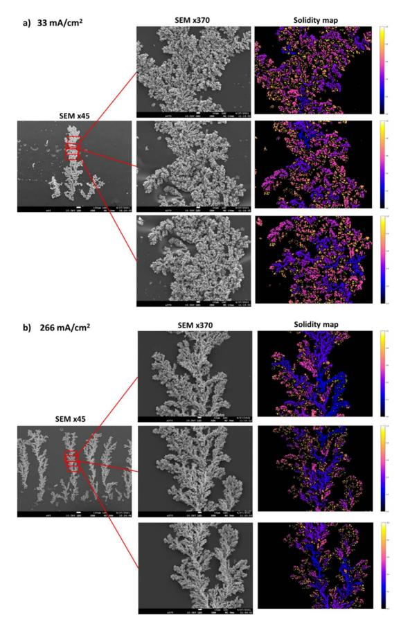
**Figure 11.** SEM images of copper branches over a significant part of their length at  $\times 370$  magnification and the corresponding solidity maps, for 33 mA cm<sup>-2</sup> in (a) and 266 mA cm<sup>-2</sup> in (b);  $c_0 = 0.5$  M. Solidity maps are obtained by image processing using python: automatic thresholding from MaxEntropy method (Kapur, pythreshold), particle detection and morphology properties (skimage).
