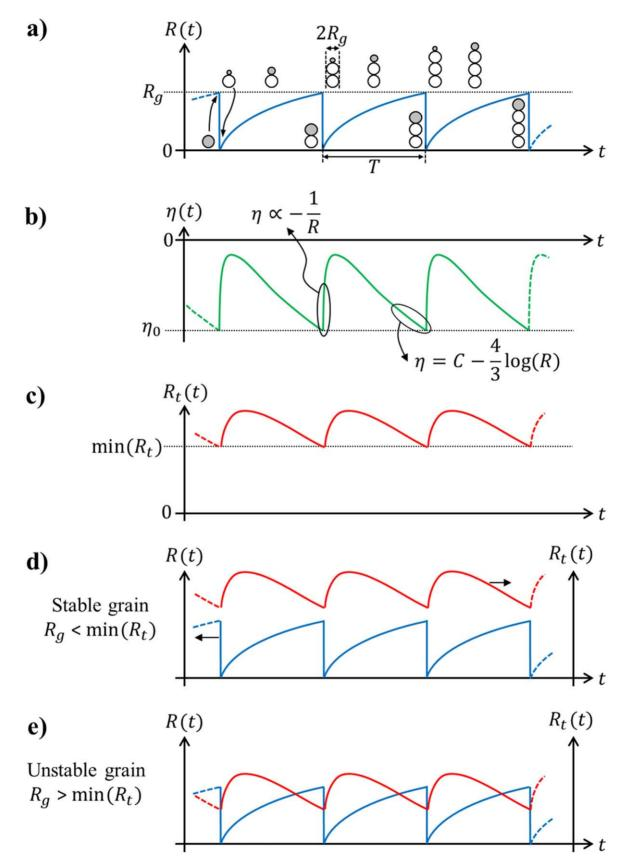
**Figure 15.** Sketches of the periodic temporal evolution of radius of a growing grain R (a), overpotential  $\eta$  (b) and threshold radius for the onset of shape instability assuming a diffusion-limited growth  $R_t$  given by Eq. 10 (c). In (a), successive nucleation/growth events are sketched, the top grain, colored in gray, is the grain which is growing. The R(t) and  $R_t(t)$  signals are plotted in the same graph for both cases stable grain (d) and unstable grain (e).
