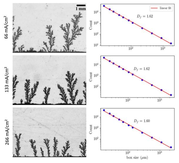
Figure 5. Left: optical images of ramified copper deposits obtained with  $c_0 = 0.5$  M and several *j* values. Right: the corresponding plots of the box counting method (ImageJ) to highlight the fractal property and to measure the fractal dimension  $D_f$  (indicated inside each graph).
