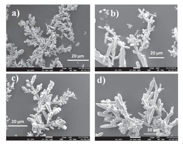
Figure 13. SEM images of silver branches (top of the branches) for the following operating conditions:  $[AgNO_3] = c_0 = 0.25 \text{ M}$ , and  $j = 33 \text{ mA cm}^{-2}$  (a),  $j = 66 \text{ mA cm}^{-2}$  (b),  $j = 133 \text{ mA cm}^{-2}$  (c) and  $j = 266 \text{ mA cm}^{-2}$  (d).
