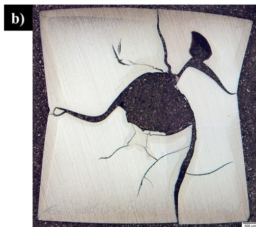
Figure 10. a) Direct sintering test of an yttria doped zirconia sample: temperatures of the upper surface of the specimen, applicator length and dissipated power as a function of time and b) axial section of an yttria doped zirconia cylinder observed by optical microscopy after a direct microwave sintering test. The central part of the specimen separated from the rest of the part during cutting.
