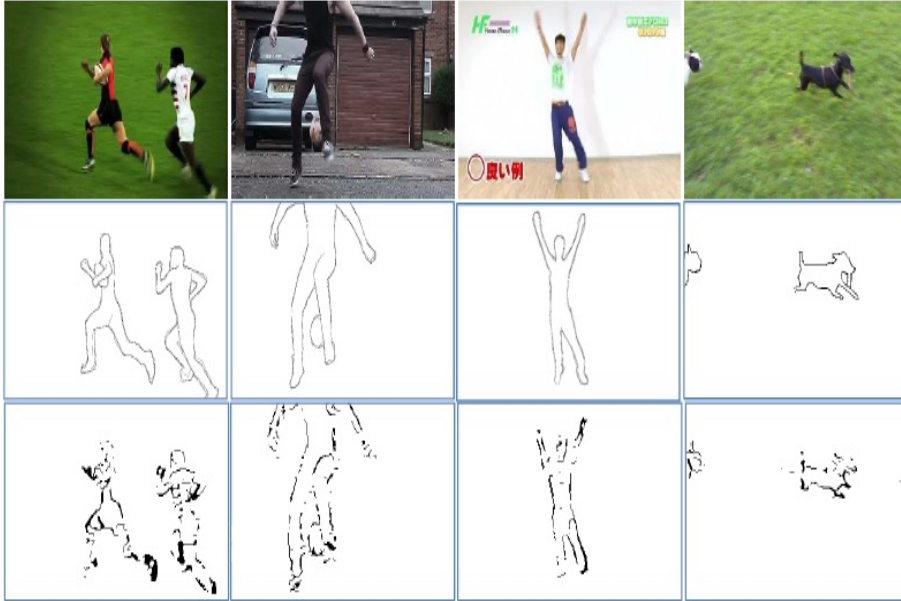
Fig. 3 Motion detection results on YMB dataset. First row shows a frame from a video sequence. Second row shows the associated ground truth frames. Third row shows the estimated motion boundaries with our proposed approach.
