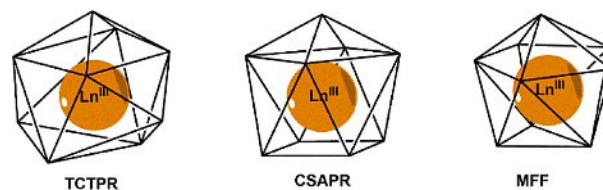
Figure 1. Graphical illustration of a tricapped trigonal prismatic (left), spherical capped square antiprismatic (middle) and muffin (right) coordination of Ln III ions.
