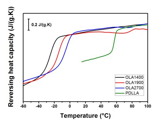
**Figure 1:** MT–DSC reversing heat capacity signals recorded in the glass transition range for amorphous PDLLA and OLAs.
