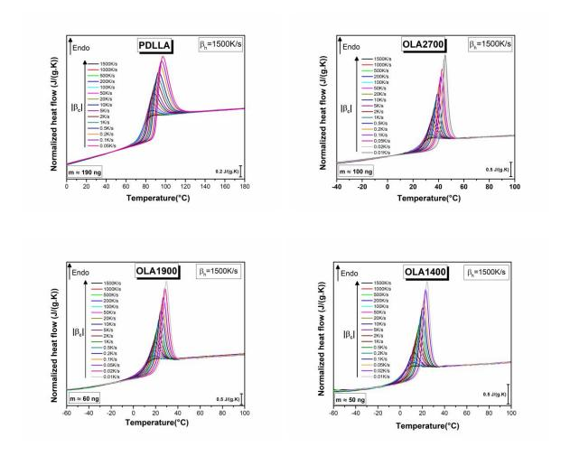
**Figure 5:** FSC normalized heat flow of amorphous PDLLA and OLAs for various cooling rate  $|\beta_c|$  (ranging from 0.01 K/s up to 1500 K/s) at constant heating rate  $\beta_h = 1500$  K/s. The sample masses have been estimating by comparing the  $\Delta Cp$  step values obtained by MT-DSC and FSC.<sup>[8]</sup>
