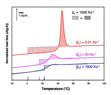
**Figure SI.2:** Principle of the area matching method used to determine the limiting fictive temperature  $T_f$  for various cooling rates  $|\beta_c|$  at constant heating rate  $\beta_h = 1500$  K/s. Dashed lines and arrows mark  $T_f$ . Dotted lines are used to show temperature dependence of Cp in glass and liquid like states.
