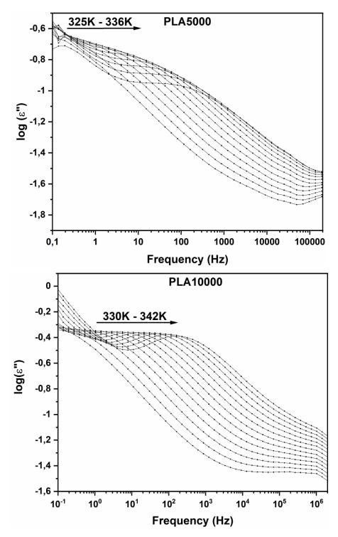
**Figure SI4**: Frequency dependence of the imaginary part of the complex permittivity  $\varepsilon$ ' at several temperatures in logarithmic scale for PLA5000 and PLA10000.
