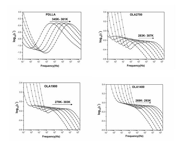
**Figure 2:** Frequency dependence of the imaginary part of complex permittivity  $\varepsilon''$  at several temperatures in logarithmic scale for PDLLA, OLA2700, OLA1900, and OLA1400.
